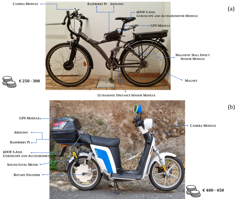
Figure 1. Raspberry-based system configurations. (a) bike; (b) scooter.
