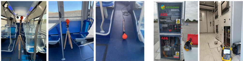
Figure 1. Measurement of magnetic field on board of the vehicle (left) and measurement system of electric quantities in the correspondence of MU and in AC/DC substation (right)
