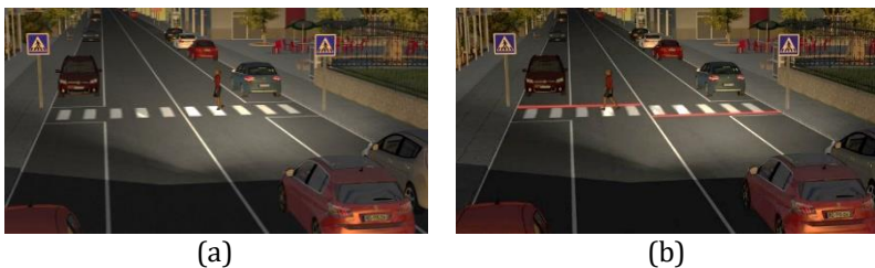
Figure 1. Crosswalks (a) without, (b) with smart red LED strips. In the smart crosswalk, the light was activated when the pedestrian stepped inside an area monitored by a set of virtual cameras.
