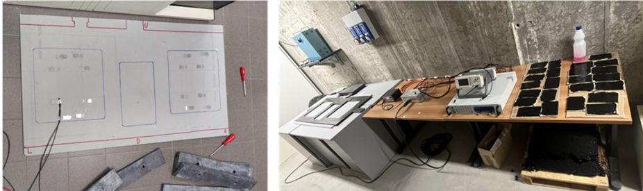
Figure 2. Preparation of one of the floors of the non-magnetic structure to support the specimens with its sensors (left) and framing of the coil with all the necessary instrumentation for its operation (right)
