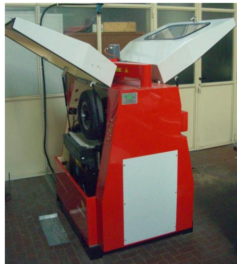
Wheel tracking test on asphalt mixes
