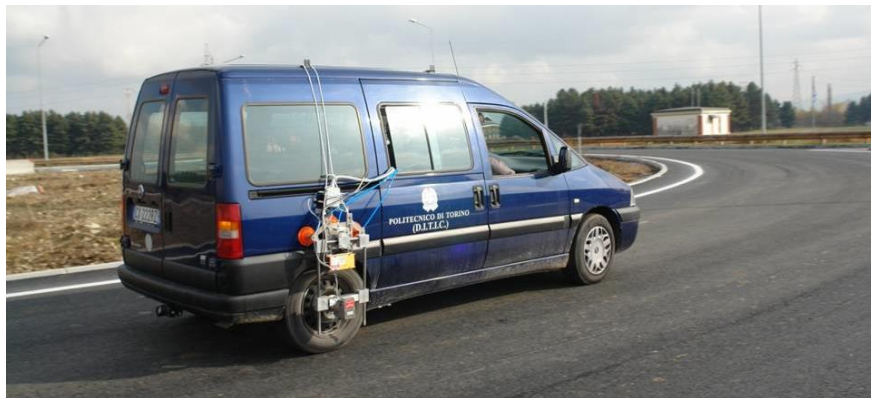
Roughness testing on pavement surfaces
