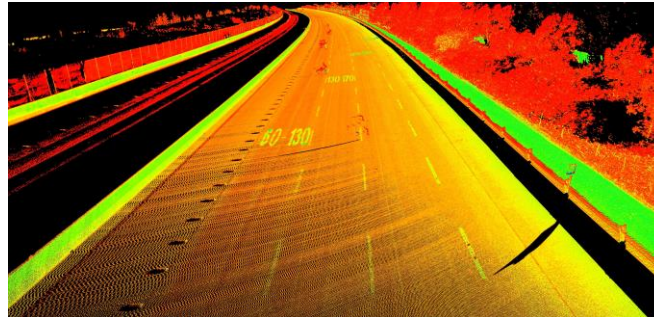
Laserscanning of pavement race tracks
