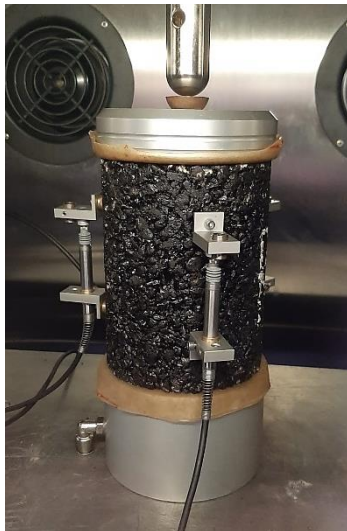
Dynamic modulus test set-up
