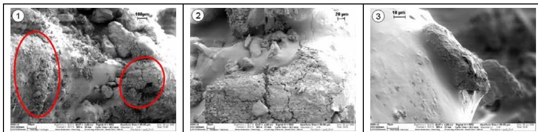
Figure 4 Dirt adhesion and development of dirt agglomerate (marked with circles) (1); enlarged image of dirt agglomerate (2); dirt adhesion on bitumen (3) [Maróthy, 2006; Kuti, 2006]
