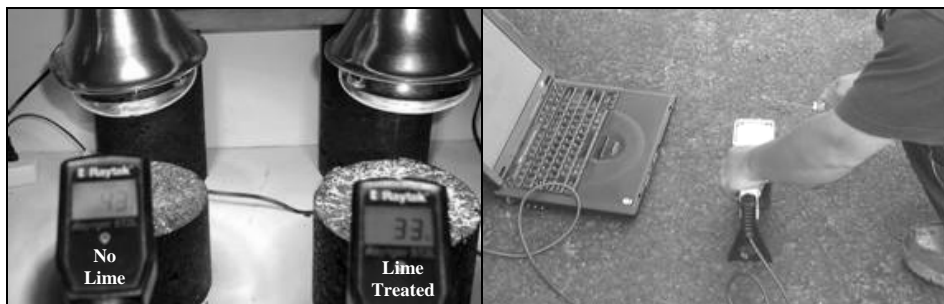
Photograph 8 Laboratory Surface Temperature Testing of Asphalt Concrete Specimens (Left) and Field Testing of Asphalt Concrete Pavement With Impact-Echo Equipment (Right)
